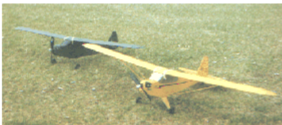
The Dawn Patrol of Cubs by Dave Jones and Eric Shultz use Goldfire motors, Master AirScrew 2:1 gearboxes, Kyosho 9x8 props and seven 1700SCRC cells. This setup brings new life to the GP Cub.
