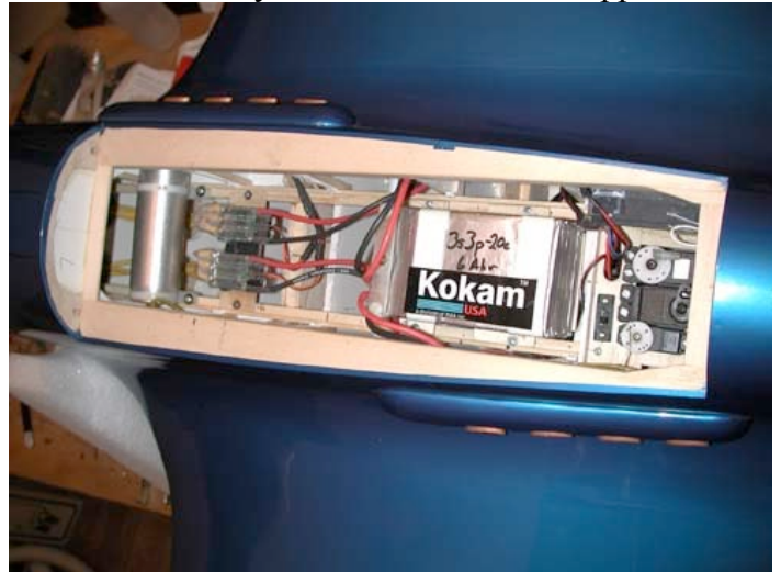
Two Castle Creation 45-amp brushless controllers and a battery of Kokam 2Ah Li-Poly Cells in a 3S3P configuration
