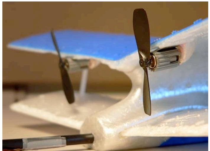
Motors control speed and direction
