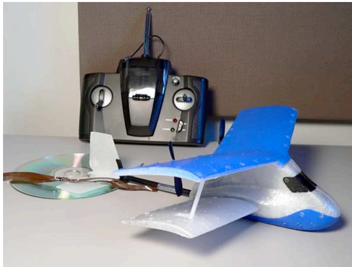
Photo shows Plane, Transmitter & CD Note the upgraded drinking straw struts!
