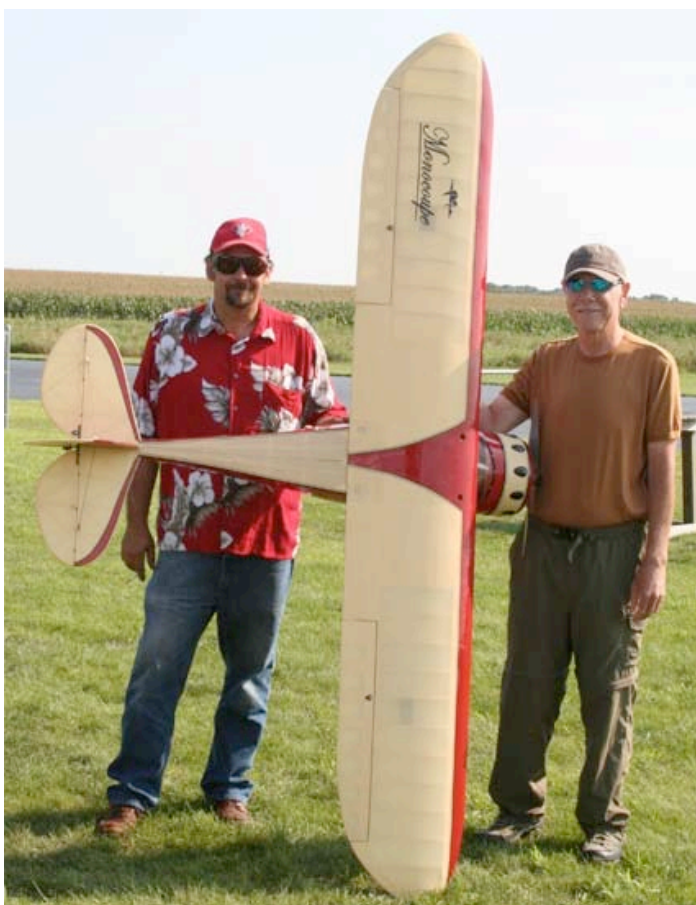
This Monocoupe uses 24 NiCads and a brushed AF 40 w/Super Box and it is still lighter than the gas version!
