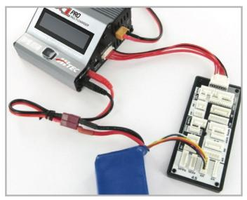
Page 16 of the manual has a VERY IMPORTANT NOTE about plugging in the Balance Adaptor to the charger. "The balance wire attached to the battery must be connected to the charger with the black wire aligned with the negative symbol (-)."
