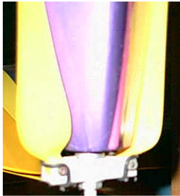
The front end of Chris's Oly 100 showing "ring washers" to aid in folding the prop.
