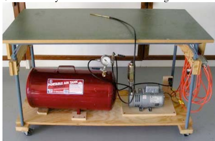
Jim's Vacuum Pump system for composite wing. About $150 in parts.
