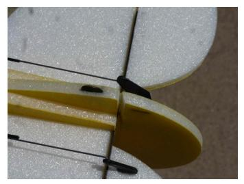
Pre-drill the holes for motor mount before attaching the mount to the fuselage with epoxy. A little right and down thrust can be can be added before the epoxy sets.
