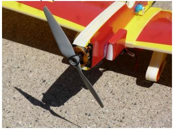
With the motor mounted, the ESC can be double sided foam taped to the bottom of the fuselage.
