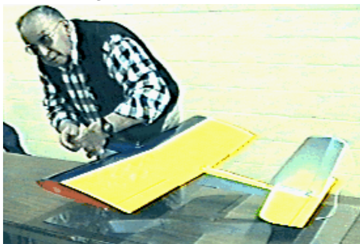
Guest Chuck Davenport shows off his original design. It has two wings, one with and one without ailerons.
