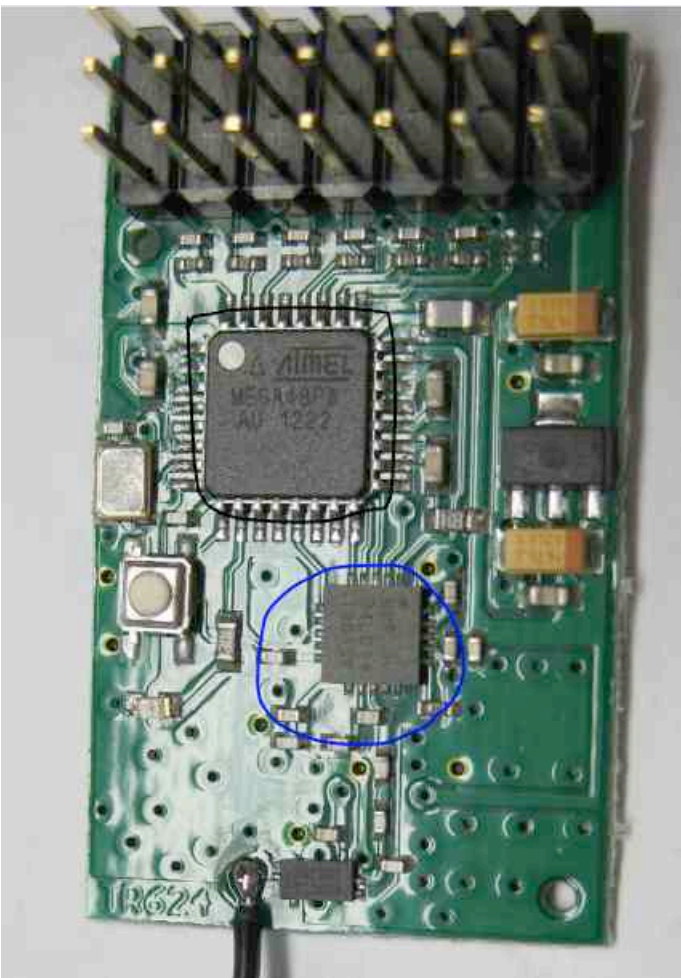
The Blue circle is the 2.4 chip. It's a Nordic nRF24L01+
