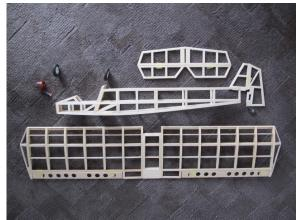
Using the plan one takes the cut strips and simply follows the layout. Then a series of spars from harder material are glued in place. The main spar is actually an "I" beam so size for size although March 2017
