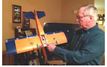
He also demonstrated the hatch and simple battery retainer of his Torpedo design.
