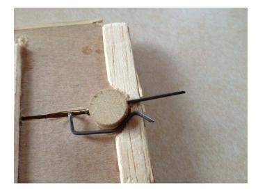
Attached are some photos of the hatch latch I use. The photos show a more compact and neater installation. The rear crossbar is not a travel stop. It is used to reinforce the 1/32 ply cover plate. The unlock stop is actually the end of the slot.
