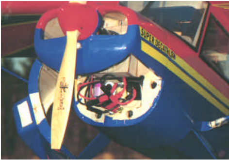
Photo #7: Cowl access to Battery pack.
