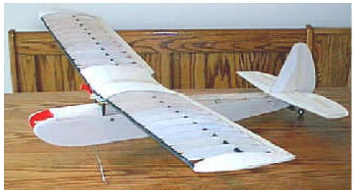
At the end of **Day 4** all covering was completed. Hinging was done while covering using Monokote style hinges, as used on all my planes. To see how I do this, check my X-250 article online. The horizontal stab and elevator become an assembly, as well as the vertical stab and rudder. It is easier to add the control horns and tailwheel strap at this time. The hatch tab and lock were added.
