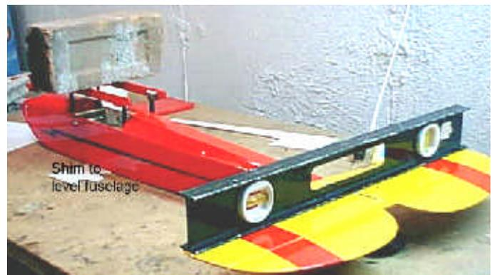
Hint 2: While gluing on the horizontal stab, if you don't have two carpenter levels to level the horizontal tail using Larry's method, use a carpenter level to level the wing
