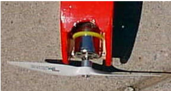
**Mod 11:** Use the original power system screws, if you have them, or purchase some DU-BRO No. 2 x ½” Socket Head Sheet Metal Screw Cat. No. 381. Use the screws to attach the “U” to the bottom of the original motor mounts and the anti-spreader bar to the top. Slide in the motor and snug them up so that the motor can’t
