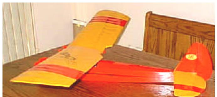
**Day 5** started with the gluing in of the canopies, carefully adjusting and gluing on the horizontal stab/elevator unit and then gluing on the vertical stab and rudder unit. Finally the Monokote hinge, already installed on the bottom of the rudder, was ironed to the fuselage, under the horizontal stab.
