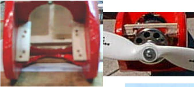
**Mod 9:** Make the front cross anti-spreader piece from plywood. I used 3/32” plywood cut to ¼” wide and glued appropriate size pieces of plywood to just retain the top of the motor. The picture shows what it
