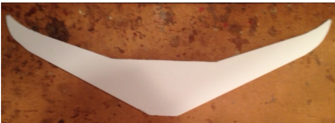
The wing planform cut out of foam board
